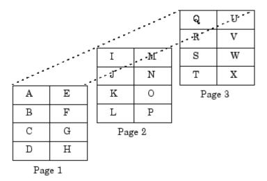
MATLAB internally represents the data for this three-dimensional array in the following order:
